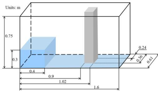
Fig. 4 Schematic diagram of the numerical dam-break tank
