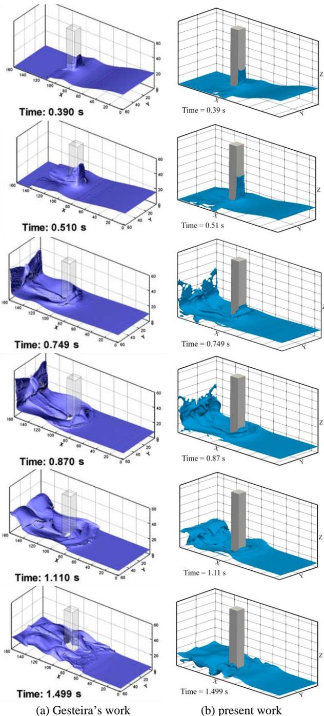
Fig. 6 Comparison of simulation snapshots of dam break on square column
