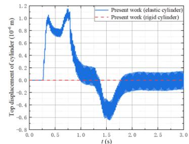
Fig. 8 Time history of top displacement of the elastic column, compared
