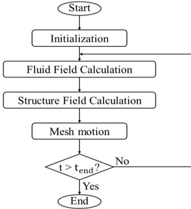
Fig. 3 Fluid structure coupling process
