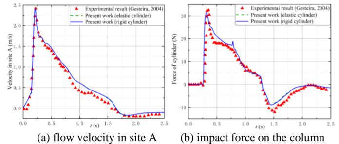
Fig. 7 Time histories of collected data in dam-break flow impacting on square column and comparisons with published experimental results
