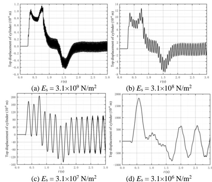
Fig. 10 Time history of top displacement of four elastic columns with different Young's modulus
